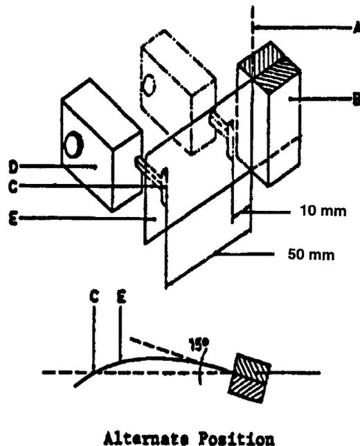
**Fig. 1.** Principle of the bending resistance tester: A. pivoting axis; B. clamping device; C. blunt knife-edge; D. force transducer with adjustable knife; E. test piece. The alternate position of the measurement head is indicated by the dashed lines.
