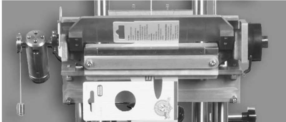
Fig. 3. Slot on the bending plate and the sample clamp bar
