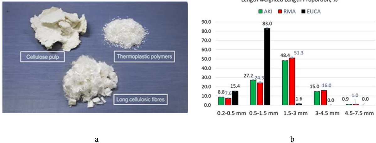
Figure 1: (a) Snapshot of fibers used in the present study; (b) Fiber length distribution of three short fiber pulps used in lab experiments. The bar color refers to the type of short fiber (green=AKI pulp, red=RMA pulp, and black=eucalyptus pulp)
