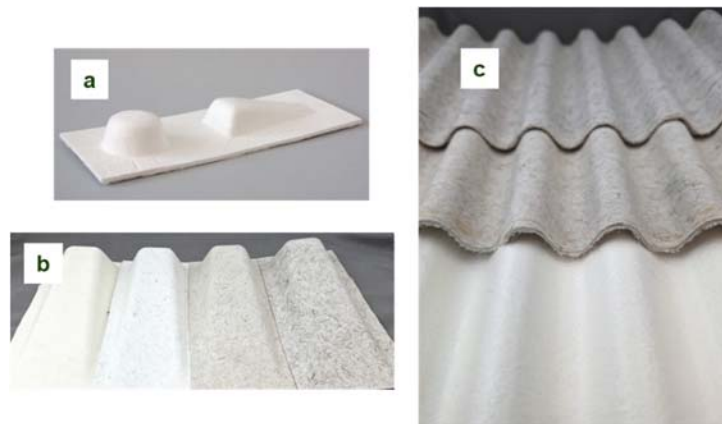
Figure 12: Thermoformed samples from lab and pilot experiments illustrating the moldability of foam-formed biocomposites (a) cup-shape from lab sample (10 mm long fiber: Tencel), (b) slope shape from lab and pilot sample (20 mm long fiber: Tencel, hemp and flax) and (c) wave shape from pilot sample (20 mm long fiber: Tencel, hemp and flax)
