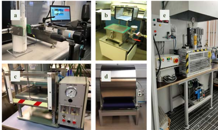
Figure 2: Composite-making procedure on a laboratory scale. (a) Foaming of fiber suspension using a mechanical mixer, (b) Sheet formation using foam-forming hand sheet mold, (c) Wet pressing, (d) Drying of samples using a drum dryer. The drying time was 4 hours at 70 °C and (e) Thermoforming using a dynamic press device.
