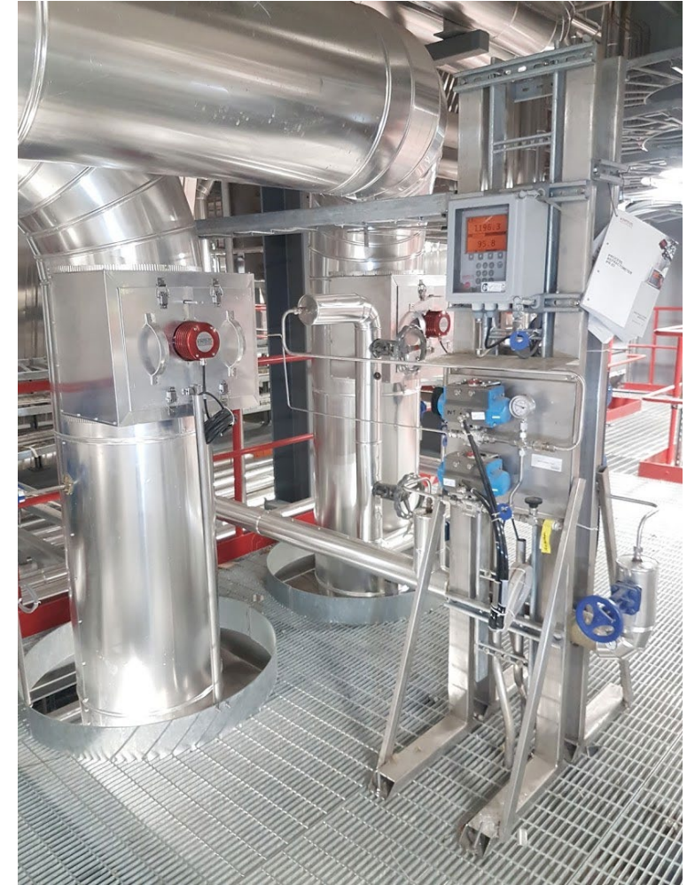
K-Patents SAFE-DRIVE™ refractometer in MetsäFibre Bioproduct Mill, Äänekoski, Finland.
