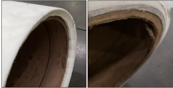
Fig. 12 Example 1 of telescoping.
