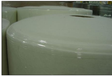
Fig. 13 Example 2 of telescoping.
