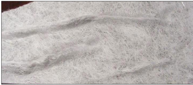
Fig. 2 Example 1 of wrinkles, ripples, folds, and creases.
