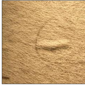
Fig. 3 Example 2 of wrinkles, ripples, folds, and creases.
