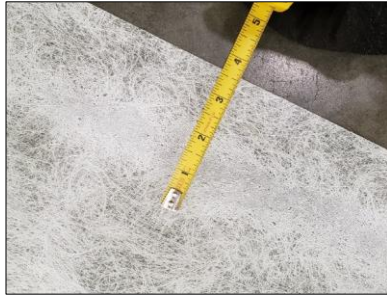
Fig. 6 Example of wet binder spot.
